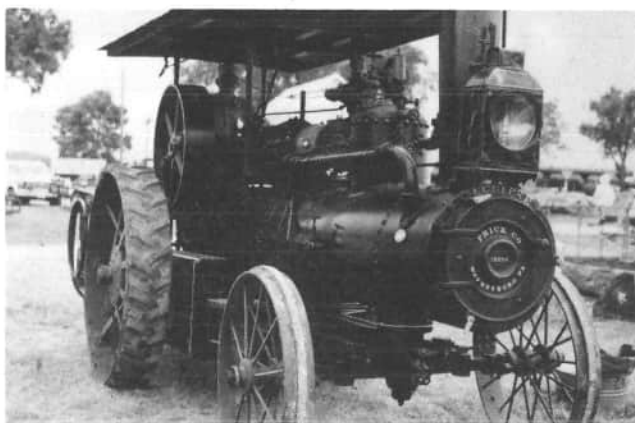
1917 Frick Steam Traction Engine; weight 7 tons, 12 horse power on draw bar, 36 horse power on belt, built in Waynesboro, PA. Engine owned jointly by Willis Lehmann, Duane Clegg, and Bill Clegg.
