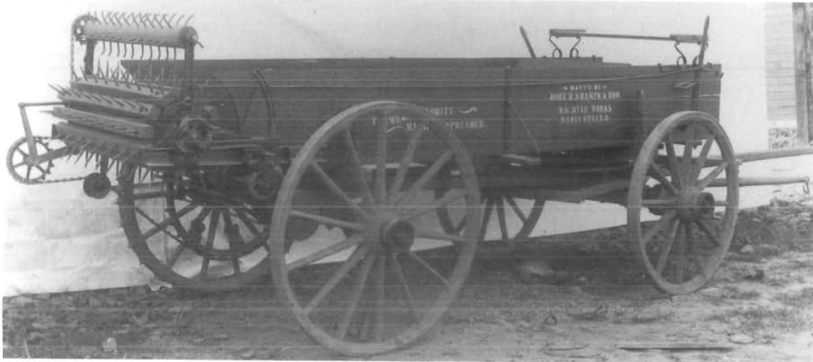
About 1898 - Manure unloader "Manufactured by John M. Kramer and Bro. Machine Works - Maria Stein, Ohio" Note - no beaters.
