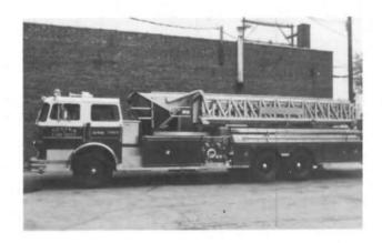
The 85 foot aerial tower quint shown above is Celina's most impressive piece of fire equipment. It was purchased from the Sutphen Fire Equipment Company, Columbus, in 1974 at a cost of \$159,113. and delivered in April, 1977.
